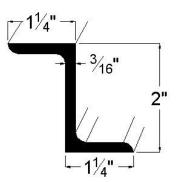
1¼" x 2" x 1¼" x 3/16" Sign support 'Z' section in a mill finish. Stocked in stronger 6105-T5 Alloy. Available in 20 ft., 10 ft. and 5 ft. lengths.
